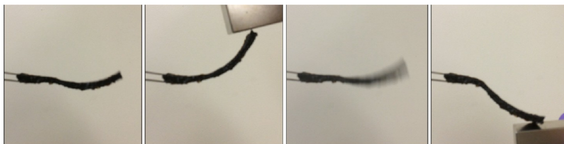
Figure 7. Bending of a hydrogel bar (length \sim 6.5 cm, 71.5 wt % water) of sample (\text{PES/Co})_{19}\text{-EO}_{800}\text{-(PES/Co)}_{19} by a neodymium magnet.
